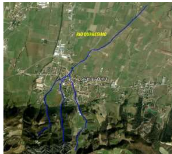
Rio Quaresimo creek, with three branches underpassing the Quattro Castella built-up area
